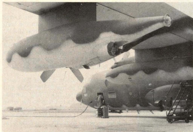
Left: Port refuelling pod of HC-130N 69-5827. Note guarded formation light for night refuelling missions. Right: Upper ramp door of the same aircraft, showing the ten ejector tubes for flares or smoke markers and the two transporter rails. Open flap on port side of the fuselage is used as an aerodynamic shield for para-jumpers and can house rocket motors for RATO
